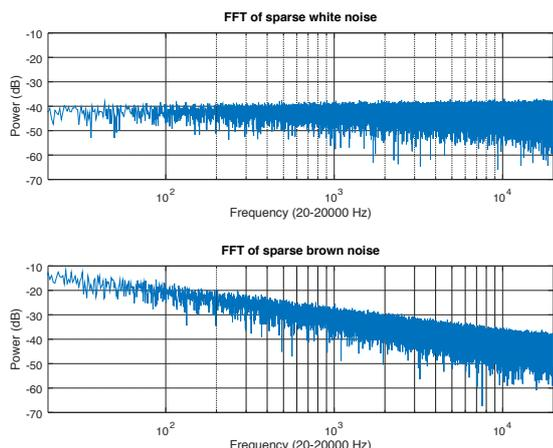
Figure 2: *Harmonic analyses of ten seconds of sparse noise.* The upper graph was produced with `sparse_noise()` from `noises.lib`. The lower graph was generated with the sparse periodic brown noise algorithm with zero periodicity. The mean event frequency  $f_0$  was 10Hz in both cases.
